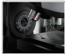
side camera shows the relationship between the lens and the workpiece, reducing the risk of collision
